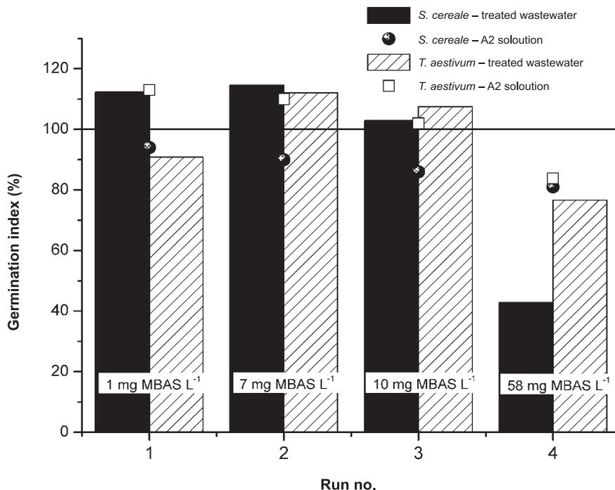
Fig. 1. The comparison of germination index (GI) calculated for cereals towards A2.
